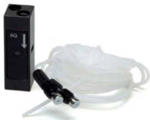
Fluorescence flow cell, 40 \mu L, 10 mm path length, supplied with inlet and outlet PTFE tubing (1.6 mm od) fitted with M6 threaded connectors, 6610023700
